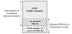
Fig. 2. Partitioning of physical channels among GSM and GPRS.
