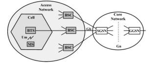
Fig. 1. Basic GPRS network architecture.
